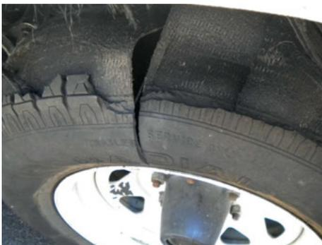
like detreads and blowouts can occur long before the tire would be expected to wear out. If the tire failure is the result of design or manufacturing defects, and the manufacturer is aware of the problem, they have an obligation to alert consumers to the potential danger.
